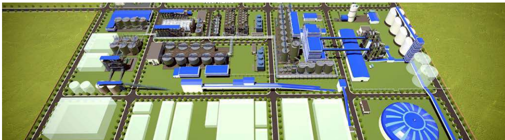
Using SYNCHRO 4D for construction simulation will save 72 construction days and CNY 57 million.
