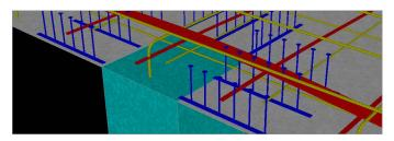
Generate realistic tendon and reinforcement layouts.
